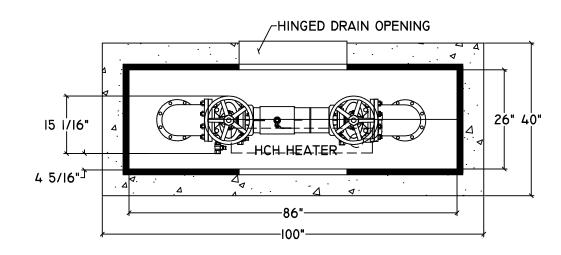
CONFIDENTIAL: THIS DRAWING IS INTENDED FOR USE ONLY BY THOSE AUTHORIZED TO RECEIVE IT. DISSEMINATION, DISTRIBUTION OR COPY OF THIS INFORMATION IS STRICTLY PROHIBITED. US PATENT 5,609,784 MODEL 400T-AL ENCLOSURE. CONCRETE PAD IS 40"W X 100"L ENCLOSURE INSIDE DIMENSIONS: ۰. ر. . م ن
