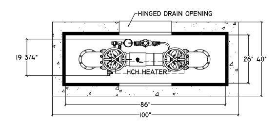
BFP DIMENSIONS FURNISHED BY WATTS ALL DIMENSIONS ARE IN INCHES DRAWING NOT TO SCALE
