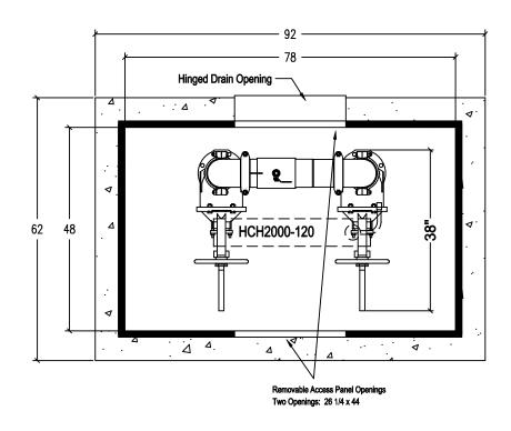
CONFIDENTIAL: This drawing is intended for use only by those authorized to receive it. Dissemination, distribution or copy of this information is strictly prohibited. US PATENT 5,609,784 MODEL 300D-AL ENCLOSURE. Enclosure inside dimensions: 48"w x 78"L x 44"H
