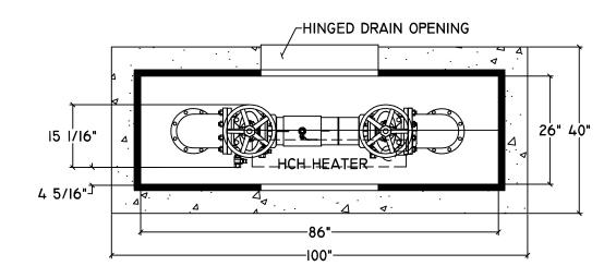
MODEL 400T-AL ENCLOSURE. ENCLOSURE INSIDE DIMENSIONS: . .
