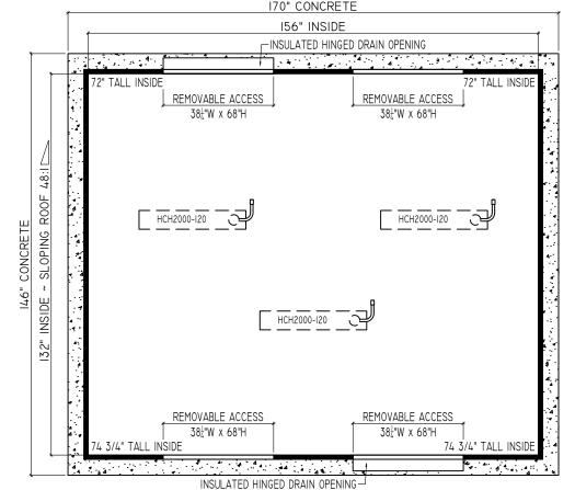
NOTE: ACCESS PANEL LOCATIONS CAN BE DETERMINED WHEN ENCLOSURE IS ORDERED
